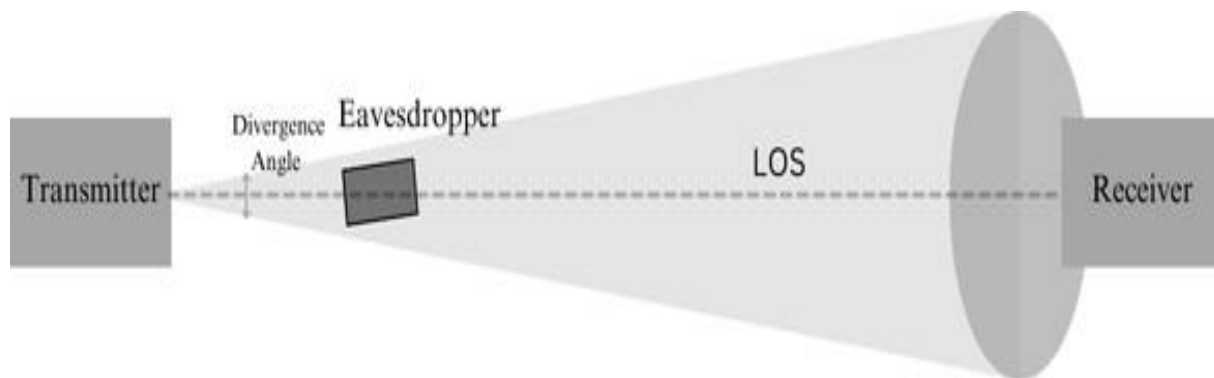
Fig 4: LoS Interception: Eavesdropper near Transmitter
